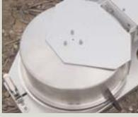
**Closed Mode:** A measurement is made once the chamber is sealed. CO<sub>2</sub> inside the large 2.7L chamber will then increase due to soil activity. The rate of soil flux is determined from the increase in CO<sub>2</sub> concentration after a user defined time interval. These measurements are simple and fast.
