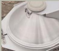
**Open Mode:** When the chamber closes ambient air is passed through the smaller 1.0L chamber at a controlled flow rate. Soil flux or rate of change is then determined at equilibrated conditions within the chamber. These measurements, although slower, are regarded as more accurate by many researchers as they are less influenced by changes within the enclosed chamber or variations in the soil structure.
